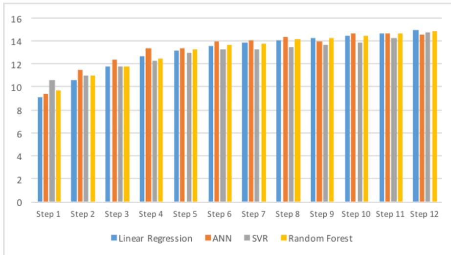
Fig. 1. MAPE 12 step ahead flow forecasting for a motorway sensor (M6)
